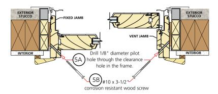
C. Apply sealant to each pilot hole drilled in the top (head) of the door frame, then insert a #10 x 3-1/2" corrosion resistant screw into each hole.
